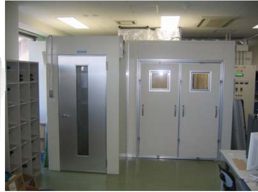
Thermostatic chamber room for environmental experiments using high-precision positioning devices and mechanisms
